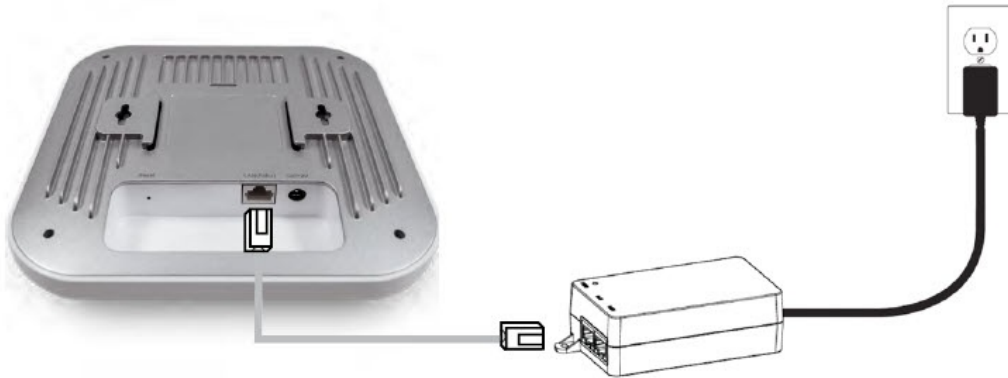
Access Point connected to PoE+ Injector
