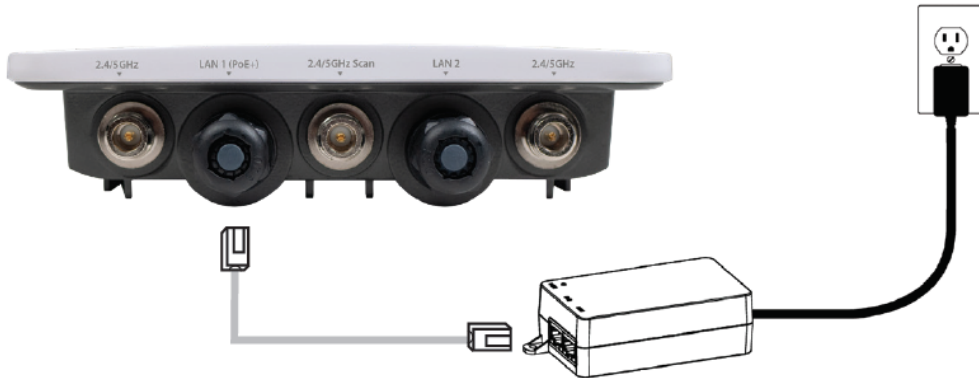
Access Point connected to PoE+ injector
